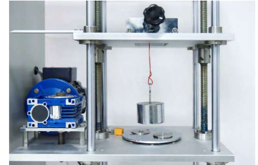
Din Rail Terminal Blocks Static Pull Test
