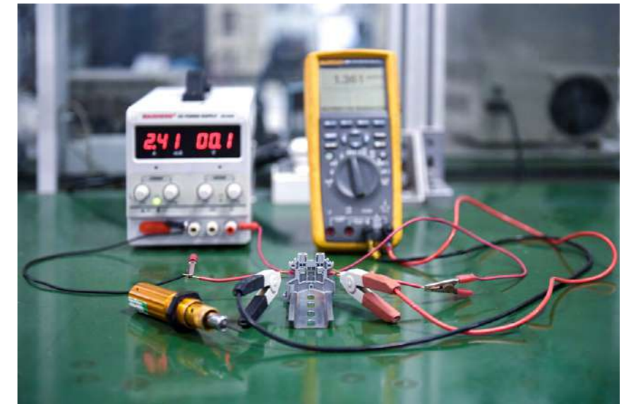
Din Rail Terminal Blocks Voltage-drop Test
