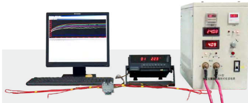
Din Rail Terminal Blocks Temperature-rise Test
