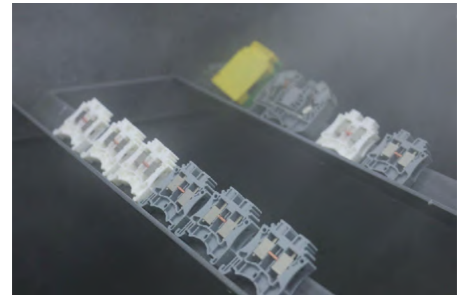
Din Rail Terminal Blocks Salt Spray Corrosion Test
