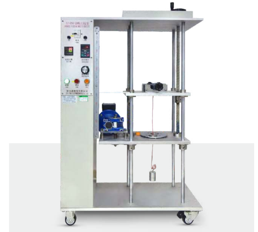
Din Rail Terminal Blocks Rotational Pull Test
